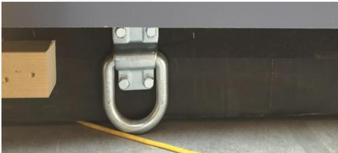
Fig. Example of brackets for securing the module to the trailer.
