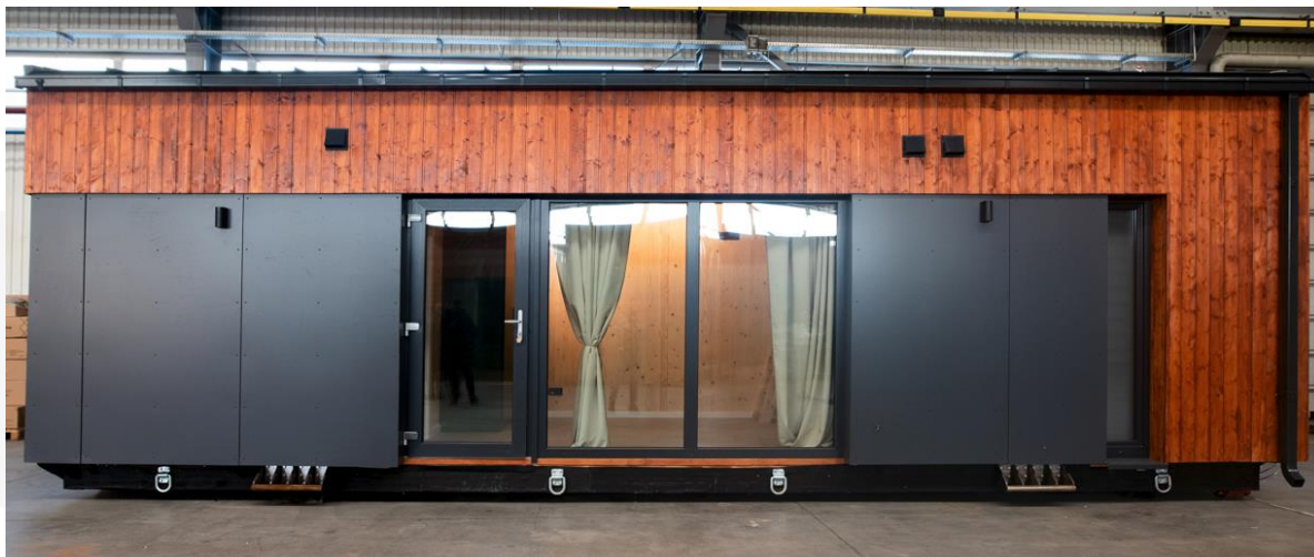
Fig. Example of brackets for securing the module to the trailer.
