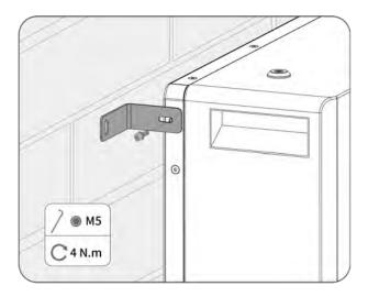
**Step 10:** Fix the L-brackets with the expansion bolts.
