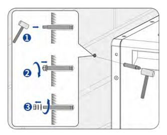
**Step 9:** Fix two L-brackets on both sides of the battery with the supplied screws(M5×10), using a Ratchet wrench (4mm) to tighten it (torque: 4 N.m).
