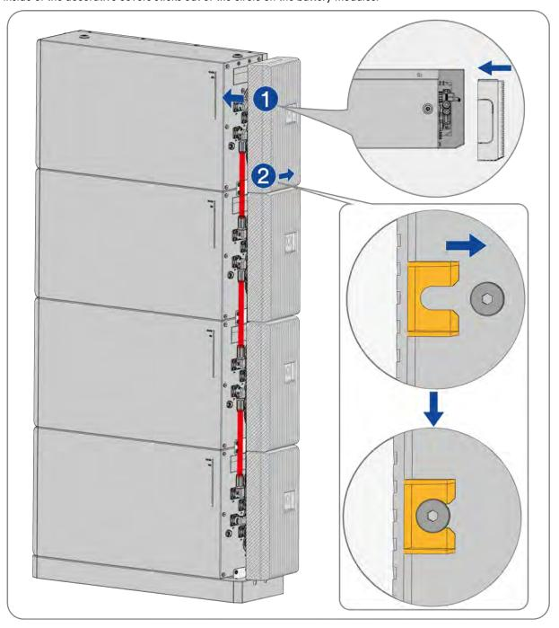
**Step 5:** Secure the decorative covers by the supplied screws(M5×16). Tightening torque: 4 N.m.
