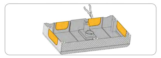
**Step 4:** Align the decorative covers with the cable area of the battery modules, cover all the cables, and push in the direction of the battery modules so that it is tight to the battery modules. Push the decorative covers backward so that the bayonet on the inside of the decorative covers sticks out of the circle on the battery modules.
