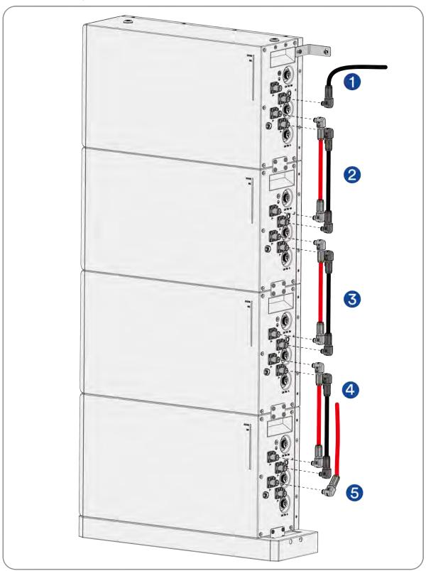
**Step 2:** Connect the "Link Port Out" of the top battery to the BMS port of the hybrid withing the supplied output communication cable(2m). Connect the "Link Port In" and "Link Port Out" between the stackable parallel batteries using the supplied parallel communication cable. Connect the bottom battery "Link Port In" with the supplied terminal resistor.
