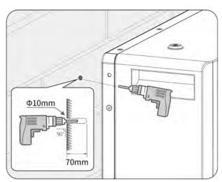
**Step 8:** Clean the dust in the hole, plug the expansion bolt into the hole, fix them with a rubber hammer, and tighten the nuts with a wrench, fix the bolt tail, and remove the nut, spring washer and flat washer and reserve them for the next step. Repeat on the other side of the battery.
