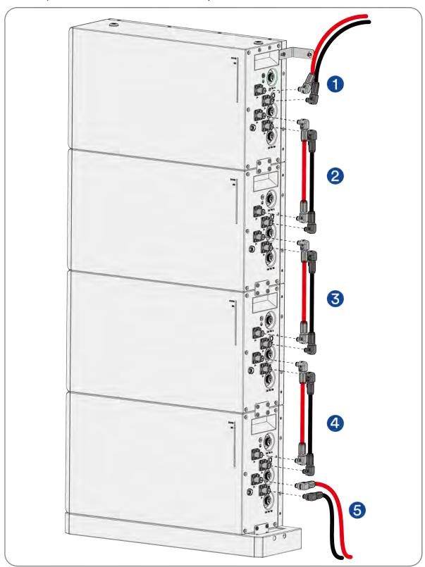
**Step 2:** Connect the "Link Port out" of the uppermost module of the battery to the battery port of the inverter using a supplied communication output cable. Connect "Link Port out" and "Link Port in" of the battery mid-layer modules using the supplied parallel communication cable. Use a supplied terminal resistor to block the "Link Port in" the lowest module of the battery.
