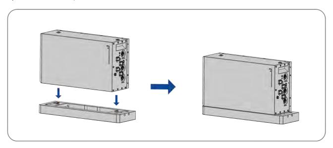
**Step 3:** Install the right anti-tipping bracket, using the module locking plate (right) to align the screw holes from above. Use four screws (M5x10) to secure the module lock plate (right), tightening torque :4 N.m.
