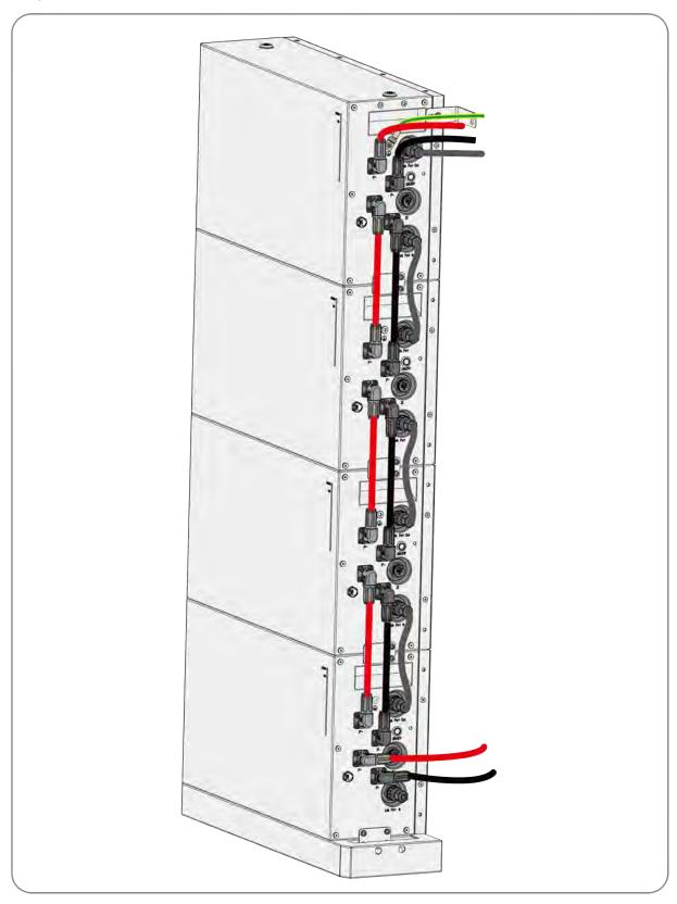
**Step 3:** Cut the cable hole according to the wiring mode.
