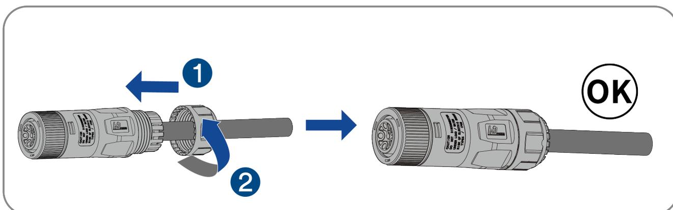
The following figure shows the sequence of the AC connector cable harness.
