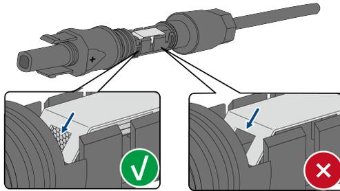
Release the clamping bracket. To do so, insert a screwdriver (blade width: 3.5mm) into the clamping bracket and pry the clamping bracket open.
