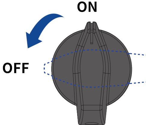
**Step 2:** Ensure that the DC switch is switched off and ensure that it cannot be accidentally reconnected.
