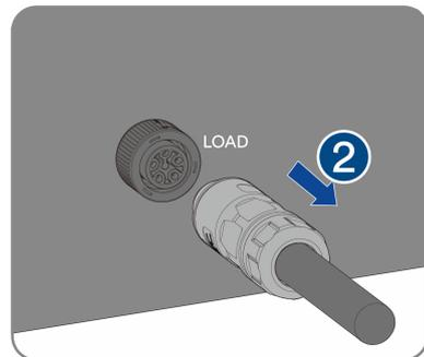
**Step 9:** Loosen and remove the Battery connector.
