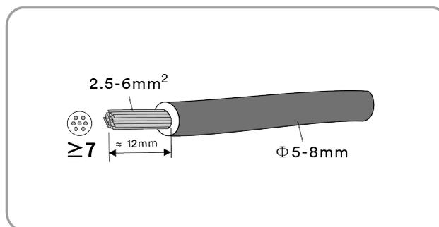
**Step 2:** Crimp the contacts with the corresponding cables. Crimping tool: PV-CZM-61100.
