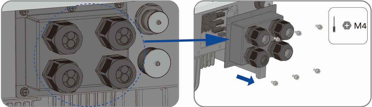
**Step 2:** Route the communication cable through the communication cover and crimp the wiring terminal.
