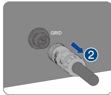
**Step 8:** Loosen and remove the EPS Load connector.
