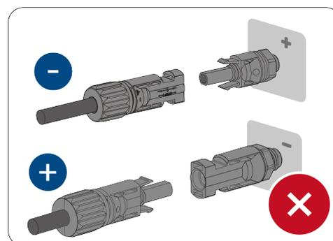
**Step 7:** Ensure that all DC connectors and the DC connectors with sealing plugs are securely in place.
