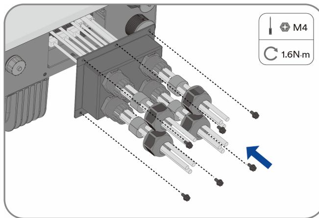
**Step 5:** Tighten the cable gland nuts.
