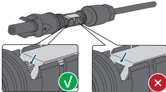
Release the clamping bracket by inserting a screwdriver (blade width: 3.5 mm) into the clamping bracket and pry the clamping bracket open.
