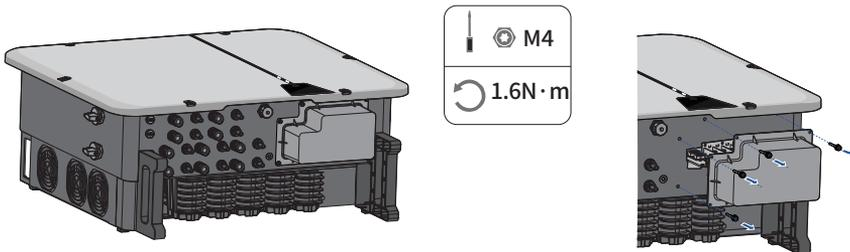
**Step 3:** Remove nut, take out the sealing ring, take out the plug, select the appropriate sealing ring according to the wire diameter, pass the cable through the waterproof connector on the AC/COM cover.
