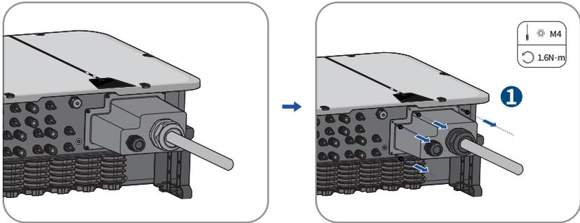
**Step 3:** Remove the nut, remove the sealing ring, remove the plug.
