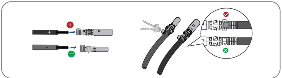
**Step 3:** Insert the cable through cable gland, and insert into the housing until it snaps into place. Gently pull the cable backward to ensure firm connection. Tighten the cable gland and onto the housing (Torque 2.5-3Nm).
