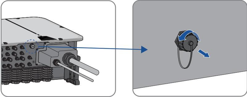
**Step 3:** Attach the Wi-Fi stick to the connection port in place and tighten it by hand with the nut on the Wi-Fi stick. Make sure the Wi-Fi stick is securely connected and the label on the Wi-Fi stick can be easily seen to allow for the scanning of the QR code during commissioning.
