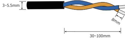
**Step 5:** Pass the cable through the gland on the AC/COM cover, and then guide the cable insert into the corresponding terminal.
