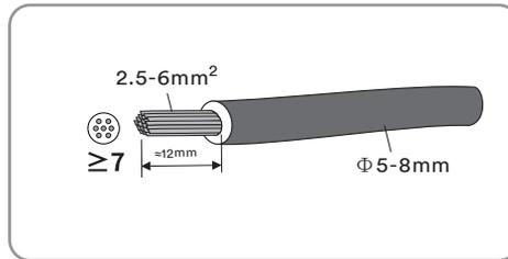
**Step 2:** Assemble the cable ends with the appropriate crimping tool.
