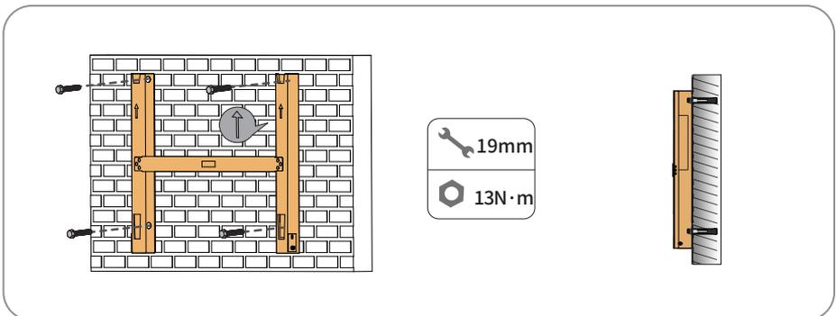
**Step 4:** Lift and place the inverter onto the mounting-bracket and ensure that the mounting flanges perfectly align with the mounting-bracket.
