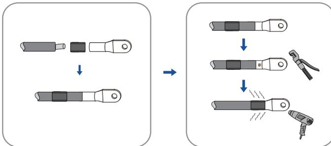
**Step 5:** Connect the wires to the corresponding terminals, use heat shrink to cover exposed metal of the AC cable.
