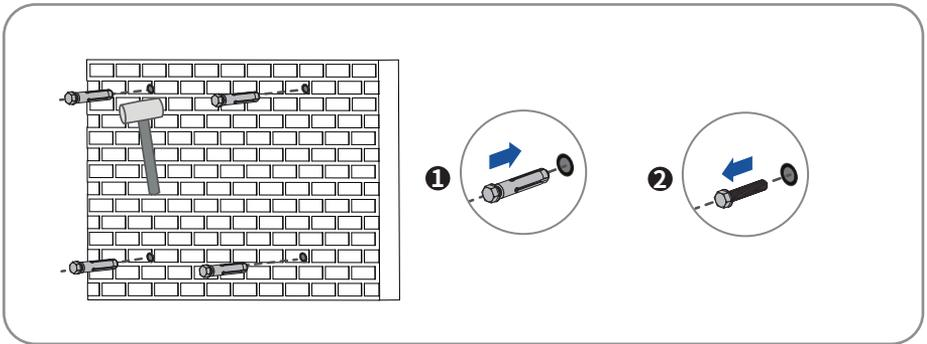
**Step 3:** Fix the mounting-bracket using the expansion bolts.
