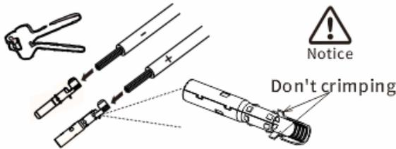
3. Insert the contact cable assembly into back of the corresponding DC plug connector. A "click" should be heard or felt when the contact cable assembly is seated correctly and tighten the swivel nut. (Torque:  $2.5\text{Nm}$ ).
