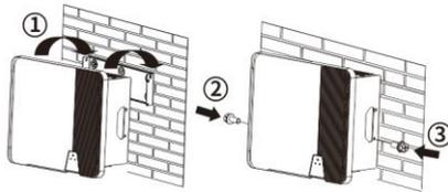
4. To protect the inverter from theft, attach the padlock provided by customer through the wall mounting bracket and the inverter.
