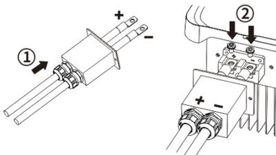
3. Tighten the battery terminal cover and cable gland nuts.
