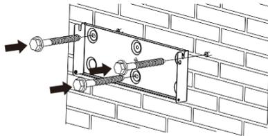
3. Hang the inverter to the wall mounting bracket. Secure the inverter to the wall mounting bracket on both sides using M5 screws.
