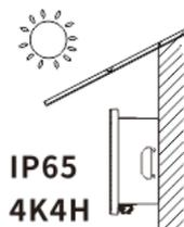
5. The mounting condition must be suitable for the weight and size of the inverter. The inverter is suitable to be mounted on solid wall that is vertical or tilted backwards (Max. 15°). It is not recommended to install the inverter on the wall made of plasterboards or similar materials. The inverter may make noise when working.
