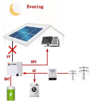
3) When there is a GRID failure, the battery supplies power to the load.
