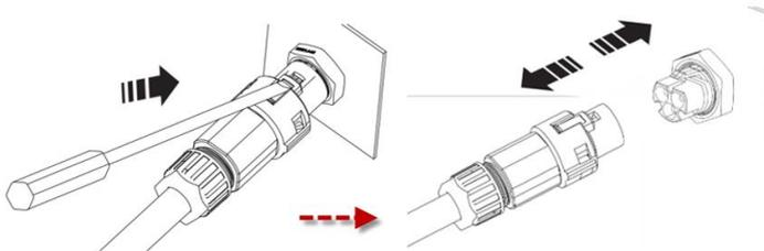
7. Release and disconnect the EPS connector. Rotate the socket element counter-clockwise to open.
