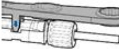
6. Release and disconnect the AC connector. Rotate the socket element counter-clockwise to open.
