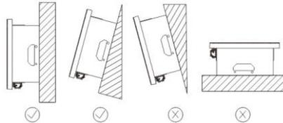
6. To ensure adequate heat dissipation, the clearances between the inverter and other objects are recommended as follows:
