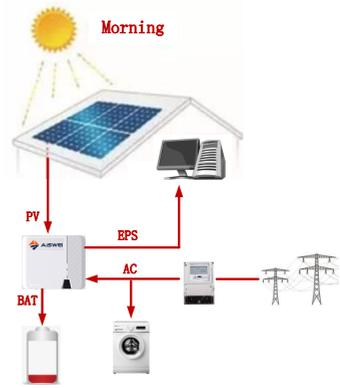
2) Under normal conditions, the battery does not discharge, Even at night.
