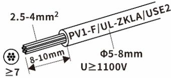
2. Crimp the contacts with the corresponding cables. Crimping tool: H4TC0001, AMPHENOL
