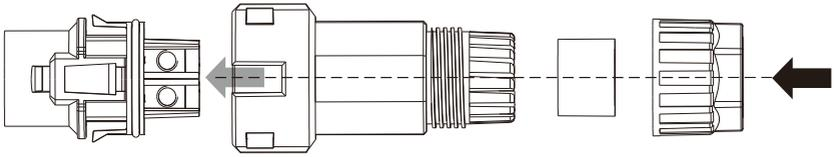
4. Insert the crimped conductors L, N and PE into the corresponding terminals and tighten the screw with a accompanied Torx screwdriver(TX 8, torque: 1.4Nm). Ensure that all conductors are securely in place in the screw terminals on the bush insert. Assemble the locking cap, threaded sleeve and swivel nut together.
