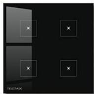
The AURUS-4S features a hardened glass touch panel with 4 capacitive buttons. These buttons consist of 4 feedback LED lights (with soft night light) and a click sound for clear and instant feedback.
