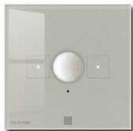
The AURUS-2 SENSE is a motion sensor for residential use: light control in hall-ways, night halls etc. The motion sensor has a horizontal viewing angle of 100 degrees and a range of 12 meter. In addition, this glass touch panel has two capacitive push buttons, a built-in temperature sensor and a light sensor which can be used independently or combined with the motion sensor function (switch light ON only when the light level is low). The trigger level can be defined in PROSOFT Suite.
