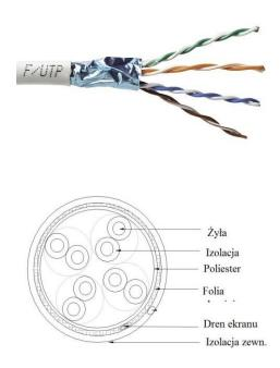
6.0mm 0.50mm ± 0.02mm; 24 AWG PCV white PF single-wire copper  $100\Omega$  +/-  $15\Omega$  for 1–100MHz 100Ω +/- 20Ω for 101-350MHz 950/km 69.00% 150MΩ/km 330pF/100m 50mm 25mm -40°C - +70 °C 0°C - +50 °C 38 kg/km cardboard box, 305m
