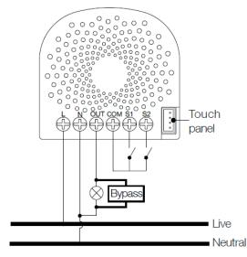
The below diagram will show you that the Nano Dimmer uses the SPDT (Single-Pole Double-Throw) switches as the external manual switch.
