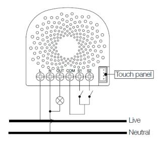
You may need to connect a small power load (E.g. a LED light or a compact fluorescent lamp) to be controlled. In this case, the Nano Dimmer may not get enough power from the AC power supply, so a bypass can be added to act as a dummy load to
