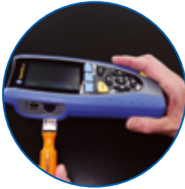
No calibration required plus replaceable RJ45 contacts
