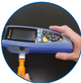
Replaceable RJ45 contacts
