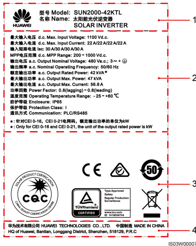
Figure 2-9 Nameplate of the SUN2000-42KTL
